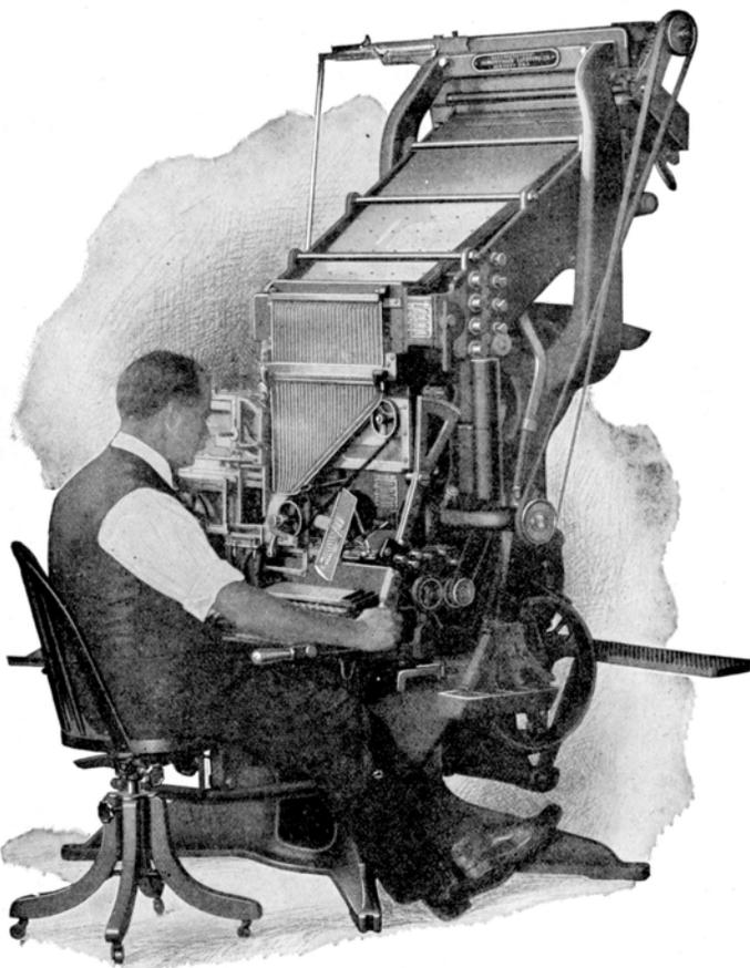
*An illustration of a typesetter using a Linotype "hot-press" metal cast printer*
